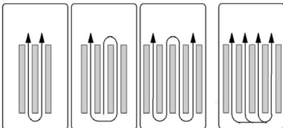
**Figure 3:** Warehouse with curve-driving S/R-machines
