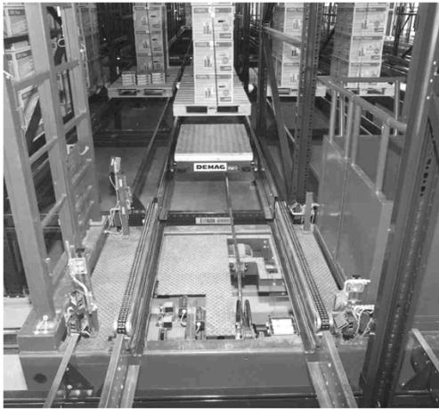
**Figure 5:** S/R-machines with channel vehicle (Mannesmann Dematic, Germany)
