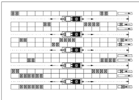
**Figure 2:** Warehouse with aisle confined S/R-machines
