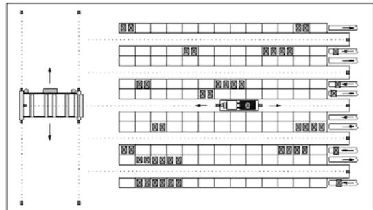
**Figure 4:** Warehouse with a shuttle device
