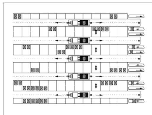
**Figure 7:** Redundant Warehouse with Access to Loading Units from Two Aisles
